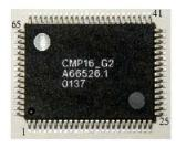
Size: 14 mm x 20 mm x 2 mm Pin pitch: 0.8 mm.
