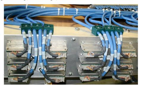
Figure 5: A view of the anode front-end boards installed on a chamber. Also shown are the AFEB-ALCT cables.
